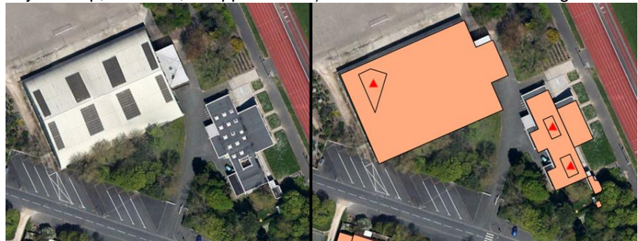
On the left side, the aerial view of roofs, and the right side the vectorial shapes in colored areas. Three artifacts overlap the building shapes in red.
