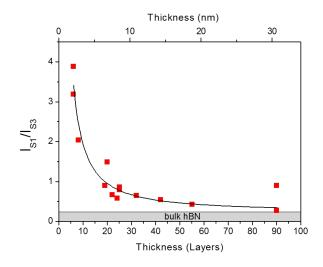
SFig. 4. Intensity ratio between S1 and S3 luminescence intensities as a function of the number of hBN layers. The signal amplitudes were measured for fixed energies at 5.898 eV/210.2 nm for the S1 emission and at 5.797 eV/213.9 nm for the S3 emission. The black line is a fit described in the text below.
