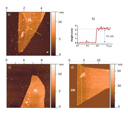
SFig. 5. AFM images of exfoliated hBN layers transferred onto a  $SiO_2/Si$  substrate composed of : a) 6L c) 8L and d) 20L. The image size unit is micrometer. Profile taken across the part of the 6L flake along the arrow is shown in b). The OC indicates a 6L thickness while AFM exhibits 3.1 nm height revealing a 1nm water layer thickness trapped between hBN and  $SiO_2$ .
