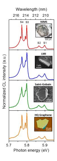
FIG. 1. CL corrected spectra of hBN bulk hBN materials in the near-band-edge region. The reference spectrum of a HPHT high quality single crystal from NIMS is compared to the chemically-grown LMI sample PDCs and the commercial hBN samples. The sample holder temperature is was 5K. All spectra are corrected from the spectral response of the detection system. In insert, typical images of the hBN materials are shown.
