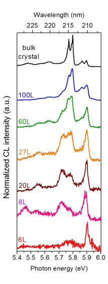
FIG. 3. Normalized CL spectra of bulk hBN and flakes of 100, 60, 27, 20, 8 and 6L obtained from the Saint-Gobain material. All spectra were corrected from the spectral response of the detection system (details in the text). The sample holder temperature was 5K.
