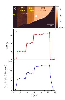
FIG. 2. a) AFM image of a mechanically exfoliated hBN flake with the dotted arrow along which was recorded the profile depicted in b) showing three distinct height steps of 9, 20 and 32 nm respectively. The profile of integrated CL signal of the S lines is plotted in c).
