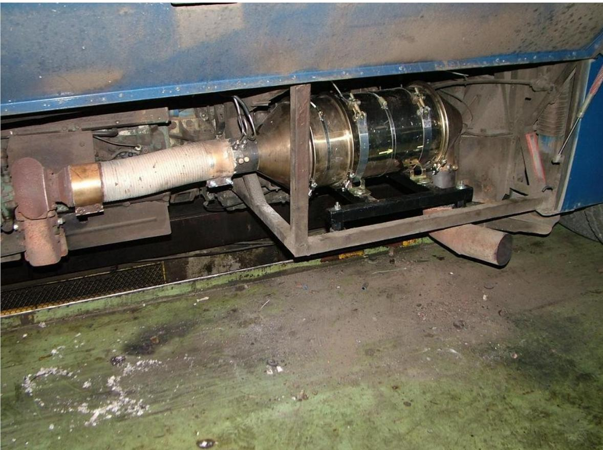
Figure 4: Rába D10UTSLL160 engine with Baumot BA1012 particle filter in a bus of Ikarus 280.40 type
