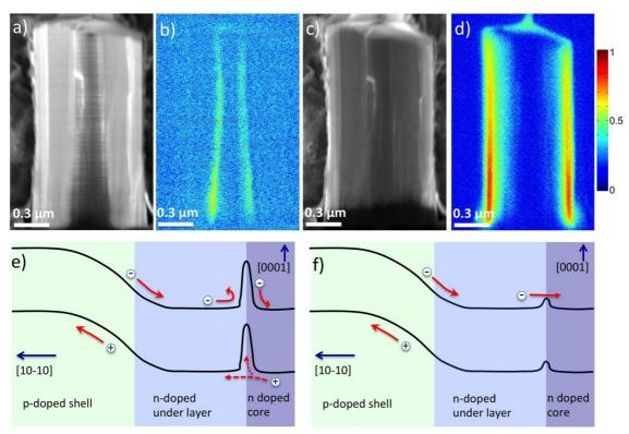
**Figure 5**. a) – Cross sectional SEM image at  $V_{acc}$ = 3 kV of a cleaved nanowire NW\_1 (the dark contrast in the nanowire core is tentatively attributed to charging effects) and b) – corresponding EBIC map before the transformation. c) and d) – same after the transformation. EBIC images of panels b) and d) are collected under the same conditions and traced in the same color scale. Schematic of the band profile before (e) and after (f) the transition.
