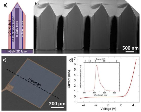
**Figure 1**. a) Schematic of the nanowire structure. b) Cross-sectional STEM image (electron beam is parallel to the <1-210> direction). c) SEM image in artificial colors of a processed 700×700  $\mu m^2$  mesa LED. The dashed line illustrates the device cleavage for cross-sectional EBIC measurements. d) I-V curve of the 300×300  $\mu m^2$  LED. Inset shows the EL spectrum for 1.8 A/cm² electrical injection.
