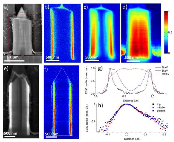
**Figure 3**. a) Cross sectional SEM image of the cleaved NW\_1 at  $V_{acc}$ = 5 kV. b), c) and d) Normalized EBIC maps corresponding to the red rectangle in panel a) collected for  $V_{acc}$  and the beam current impinging the sample of (b) – 2 kV, 0.4 nA, (c) – 5 kV, 0.5 nA and (d) – 10 kV, 0.9 nA. e) Cross sectional SEM image of the cleaved NW\_2 at  $V_{acc}$ = 2 kV. f) Corresponding EBIC map collected for  $V_{acc}$ = 2 kV and beam current 0.4 nA. The dashed line
