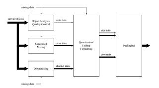
Fig. 1: Multichannel object-based audio encoder
