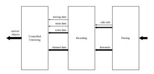
Fig. 2: Multichannel object-based audio decoder
