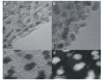
Figure 2. a, b HRTEM images of Pt/CFs and SnO<sub>2</sub>/Pt/CFs before cyclic voltammetry. c, d STEM images of SnO<sub>2</sub>/Pt/CFs in bright and dark field.
