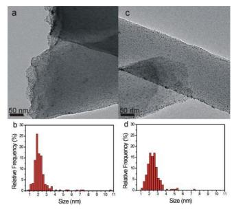
Figure1. a, c) TEM images and b, d) particle distribution obtained from TEM analysis of a,b) Pt/CFs, c, d) SnO<sub>2</sub>/Pt/CFs before cyclic voltammetry.
