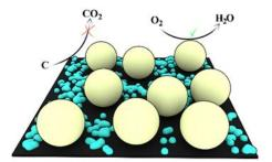
Figure 5. Schematic representation of the SnO<sub>2</sub>(blue)/Pt(yellow)/CFs (black) surface.
