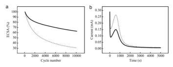
Figure 6. a) ECSA of Pt/CFs (dotted line) and SnO<sub>2</sub>/Pt/CFs (full line) calculated from cyclic voltammetry at 50 mV/s in a N<sub>2</sub> saturated 0.5 M H<sub>2</sub>SO<sub>4</sub> solution every 100 cycles performed at 100 mV/s. b) Oxidation/corrosion characteristics for Pt/CFs (dotted line) and SnO<sub>2</sub>/Pt/CFs (full line) at 1.4 V/RHE.
