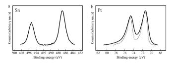
Figure 3. XPS spectra of SnO<sub>2</sub>/Pt/CFs (full line) and Pt/CFs (dotted line). High resolution scans across a) the Sn 3d and b) Pt 4f edges, respectively.
