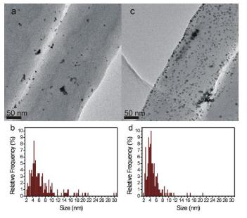
Figure 7. TEM images a,c) and b,d) particle distribution from TEM analysis of a,b) Pt<sup>5%</sup>-CFs and c,d) SnO<sub>2</sub>-Pt<sup>5%</sup>-CFs after 10,000 potential cycles.
