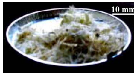
Figure 3 Appearance of shredded SMC.
