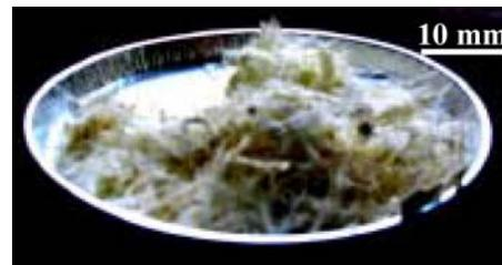
Figure 3 Appearance of shredded SMC.
