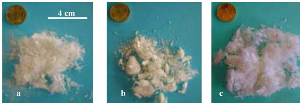
Figure 2 Appearance of the shredded SMC<sup>mod</sup> before partial solvolysis (a) and after a 3 h solvolysis et 200 $^\circ\text{C}$  with continuous stirring (b) or without stirring after moistening (c).
