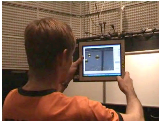
Utilization of the L-Scanner interface for controlling spatialization other a wave field synthesis restitution system
