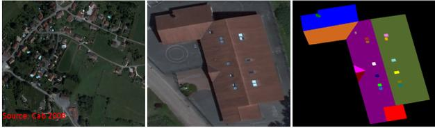
Fig. 1. Objective of the segmentation process. (left to right: an ‘‘orthophotoplan’’ image, zoom of a roof, ground truth image segmentation).
