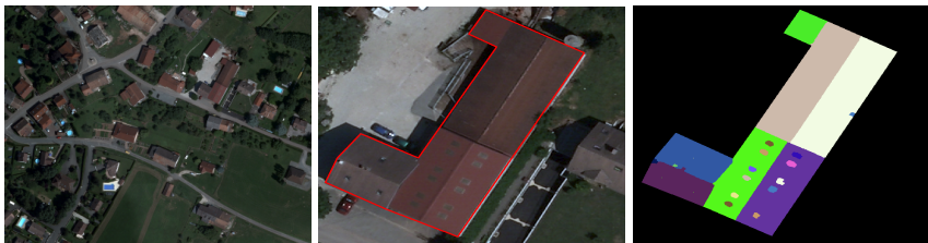
Fig. 1. Example of “orthophotoplan” image (left to right: an “orthophotoplan” image, a zoom of roof, the segmented image).
