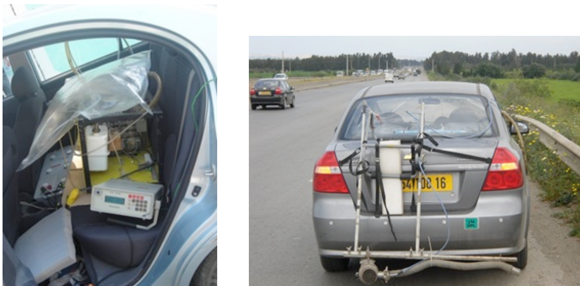
Fig. 2 Instrumented vehicle with the mini-CVS measurement system.
