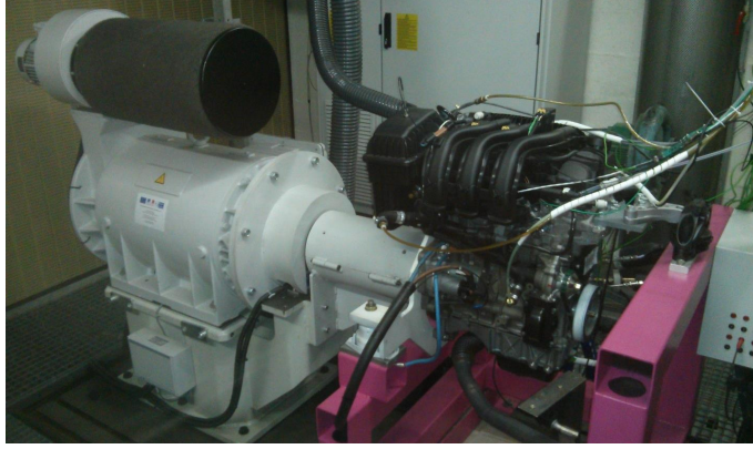
Figure 8: Test bench with the high-dynamics generator (left, in white) and the engine (right) on the chassis (right, in pink)
