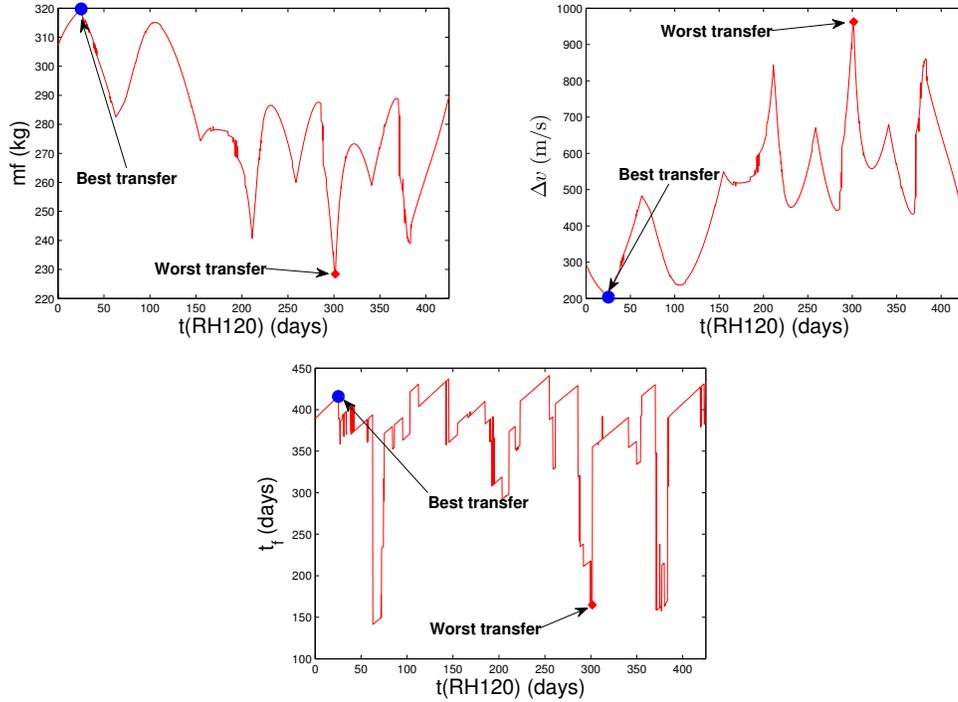
Figure 9: Evolution of the final mass (top left), of the  $\Delta v$  (top right) and transfer duration (bottom) from the Halo orbit around  $L_2$  with respect to rendezvous points on the orbit of  $\text{RH}_{120}$ .
