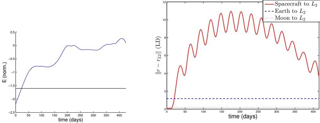
Figure 5: Evolution of the energy (left) and of the Euclidean distance to the  $L_2$  Libration point (right) for  $RH_{120}$ . For energy, the horizontal line represents the energy of the Halo periodic orbit around  $L_2$  which is about -1.58.
