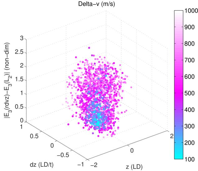
Figure 13: Characterization of 1,000 simulated rendezvous transfers from  $L_2$ .
