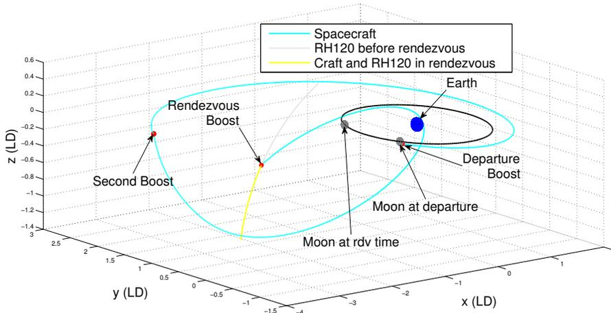
Figure 12: Best 3 boost Sun-perturbed rendezvous transfer to RH<sub>120</sub> from a Halo orbit around  $L_2$  in inertial frame, with transfer departure after RH<sub>120</sub> detection.
