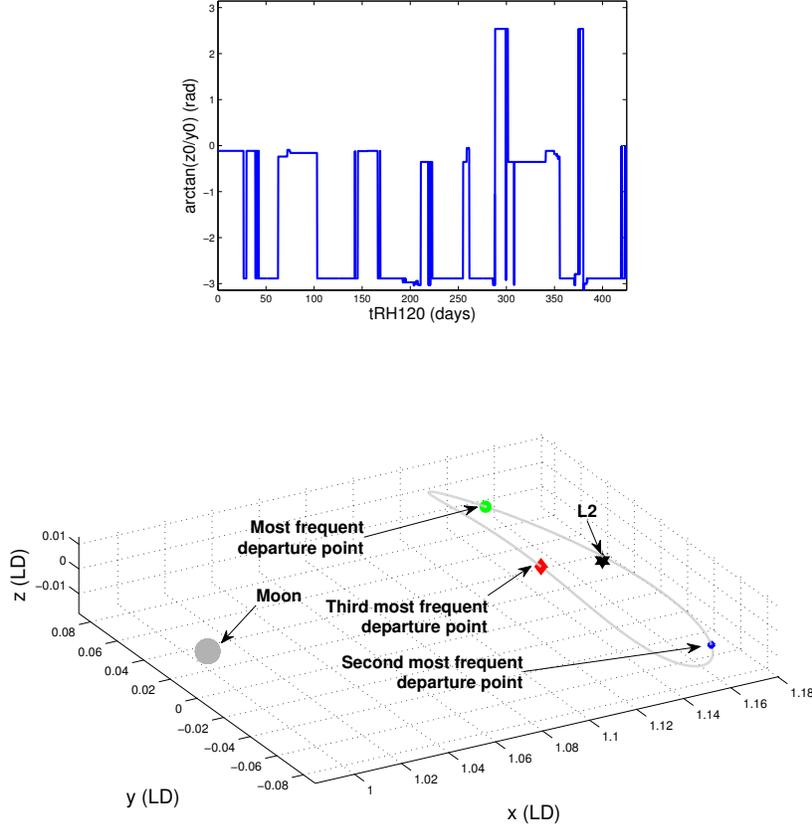
Figure 10: The top picture represents the evolution of  $(y, z)(0)$  argument with respect to time of rendezvous on  $RH_{120}$ . The bottom picture represents the three most frequent departure points on the initial Halo orbit.
