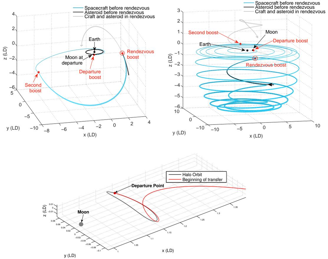
Figure 6: Best 3 boost rendezvous transfer to  $RH_{120}$  from a Halo orbit around  $L_2$ : Inertial Frame (left). Rotating Frame (Right). Bottom: zoom on the start of the departure from the Halo orbit (rotating frame).
