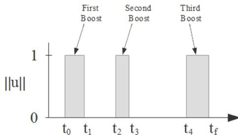
Figure 3: Control function modeling thrust impulses over time.
