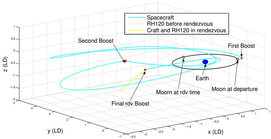
Figure 11: 3 boost rendezvous transfer to  $RH_{120}$  from a Halo orbit around  $L_2$  in inertial frame, using the CR4BP. Departure 135 days after June 1<sup>st</sup> 2006, arrival 255 days later.
