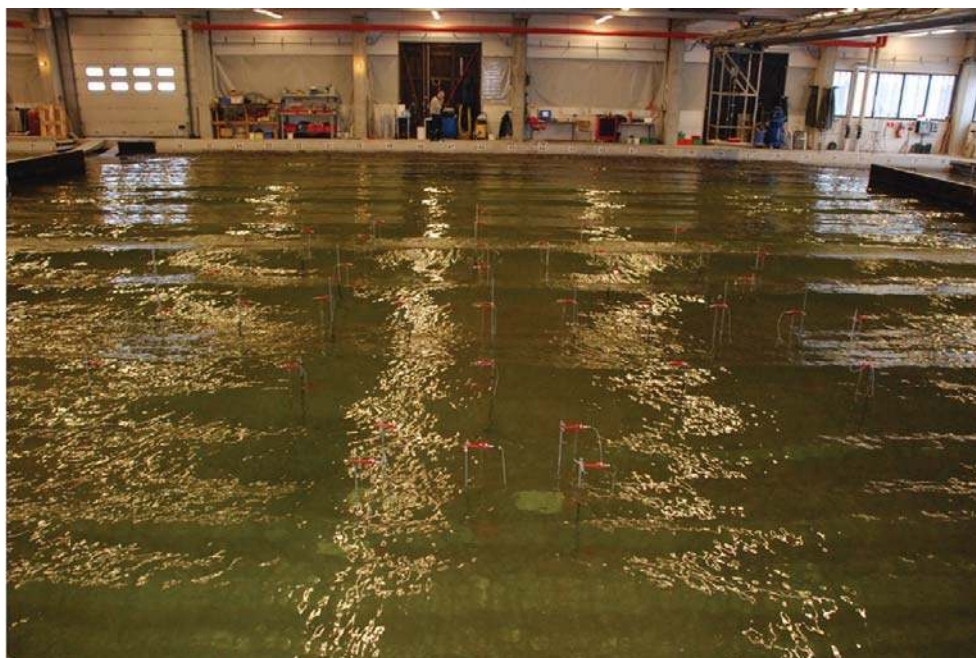
FIG. 1. Shallow Water Wave Basin at DHI (Hørsholm, Denmark). View from a location behind the wave generator, while taking wave height measurements (sea-states characterization) using a network of resistive wave gauges in the empty wave basin.
