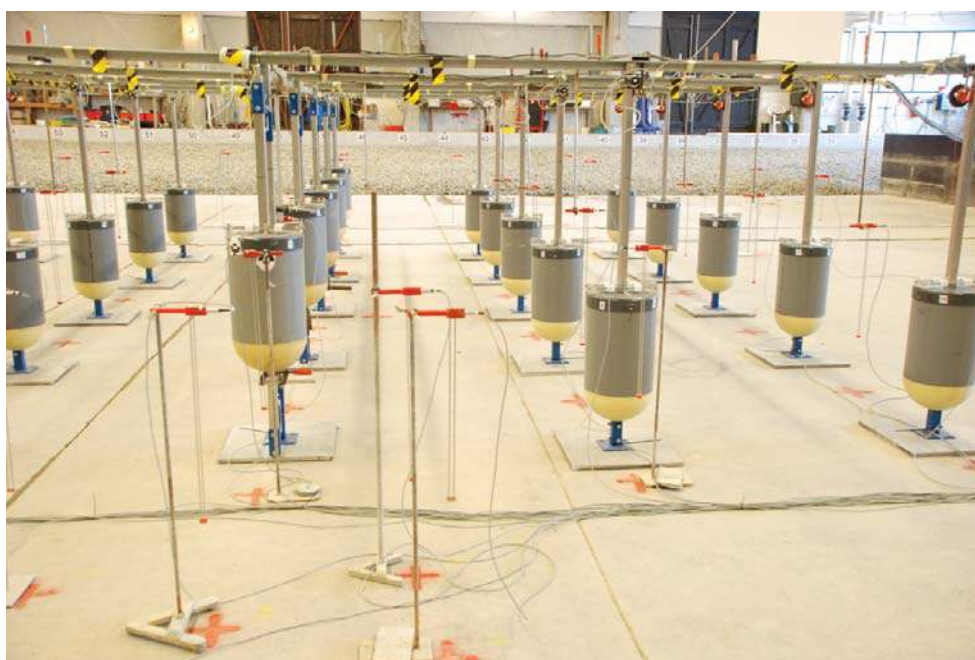
FIG. 3. The support structures for the WEC arrays.
