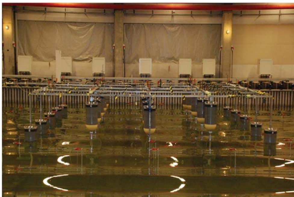
FIG. 6. A 10-WEC 2-column array (WECs #21–#25 and WECs #16–#20) under regular waves with \theta = 0^\circ . The other 15 WEC units are held stationary above the water surface. View from behind the wave absorbing beach.
