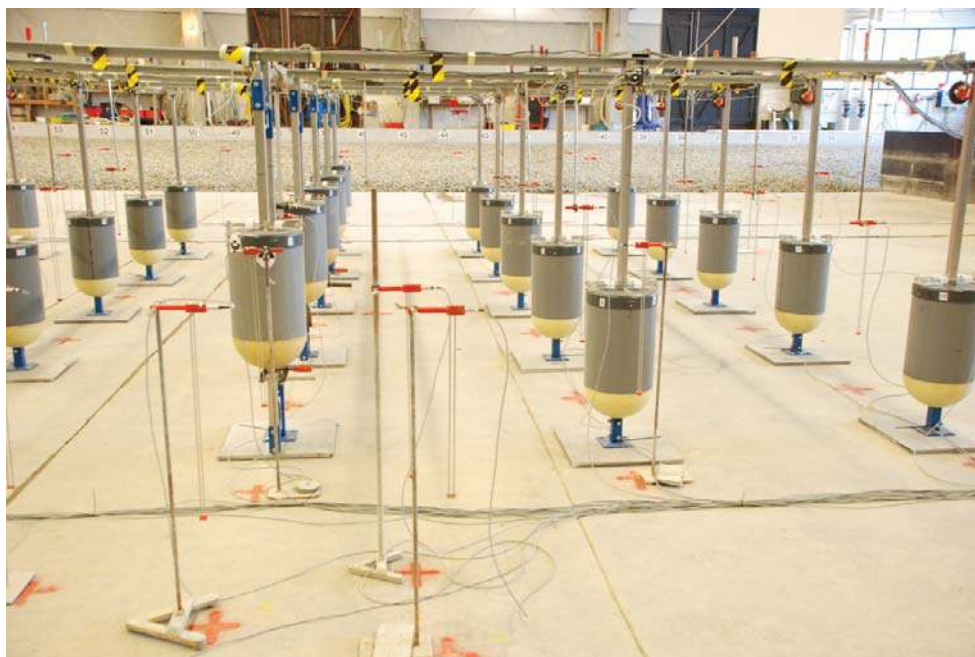
FIG. 3. The support structures for the WEC arrays.
