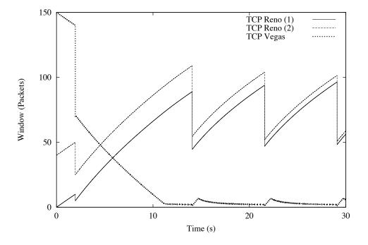
Figure 13: Competition between TCP Reno and TCP Vegas
