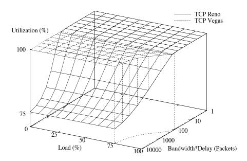
Figure 10: Utilization of the available bandwidth
