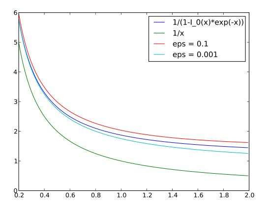
Figure 1: The function  $\frac{1}{1-\Gamma_0}$  (blue curve) compare to its classic Padé approximation 1/x (green curve) and the new approximations with  $\varepsilon = 0.1$  (red curve) and  $\varepsilon = 0.001$  (cyan curve).
