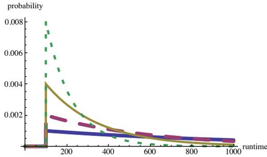
**Fig. 2** For an exponential distribution, here in blue with  $x_0 = 100$  and  $\lambda = 1/1000$ , simulations of the distribution of  $Z^{(n)}$  for  $n = 2$  (pink),  $n = 4$  (yellow) and  $n = 8$  (green).
