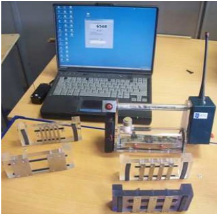
Figure 10. Devices used for obtaining the NDT data.
