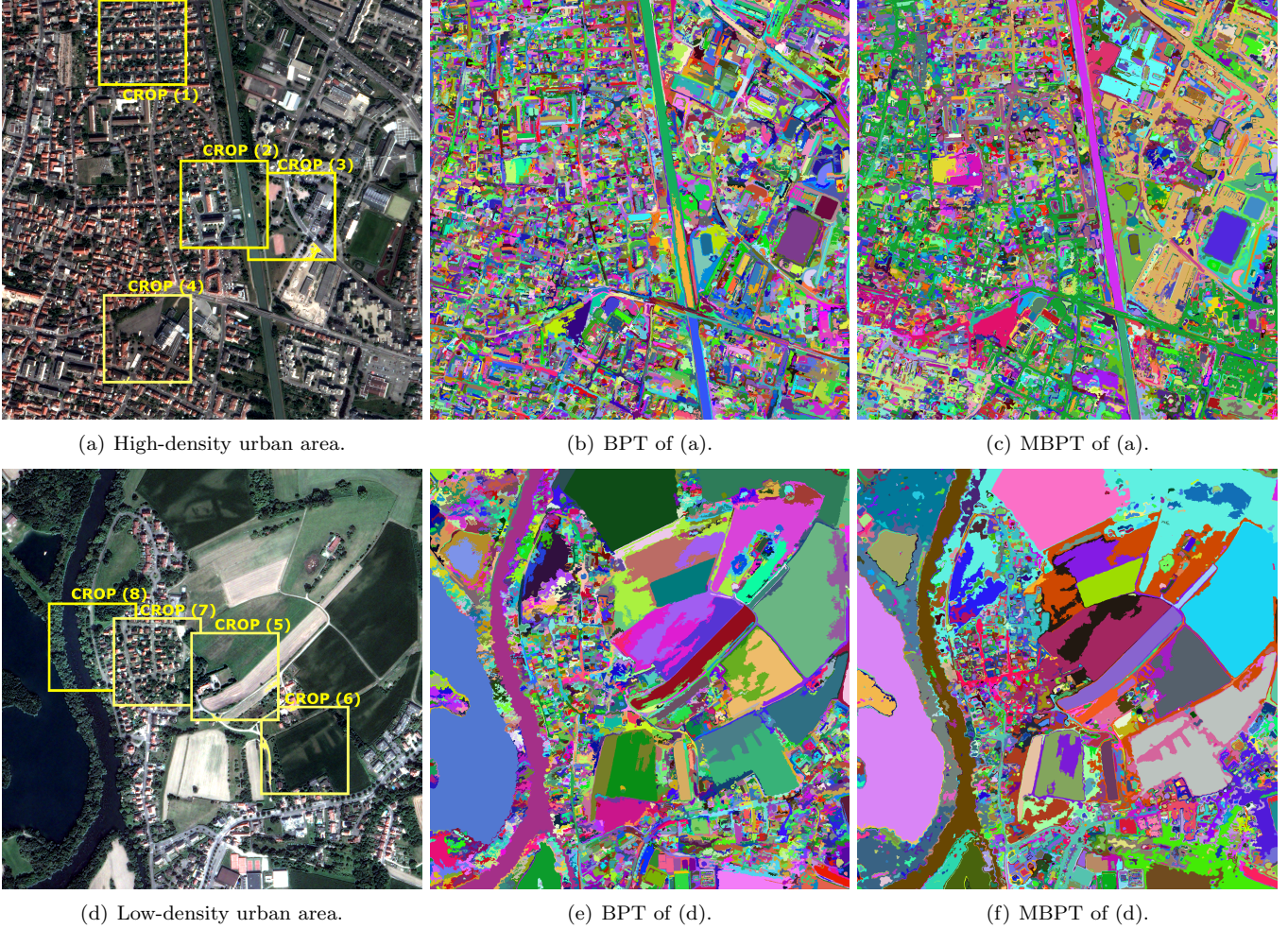
Figure 6: (a, d) Illustration of two very-high spatial resolution satellite images ( 2000 \times 2000 pixels) at a spatial resolution of 60 cm sensed by the PLÉIADES satellite and covering different geographical areas. (b, resp. e) Segmentation result from a cut containing 23500 regions (resp. 5000 regions) performed on a “standard” BPT of (a, resp. d). (c, resp. f) Segmentation result from a cut containing 23500 regions (resp. 5000 regions) performed on a MBPT of (a, resp. d) using four features: the colour intensity, the region elongation, NDVI and NDWI values \{W_{colour}, W_{elong}, W_{ndvi}, W_{ndwi}\} .
