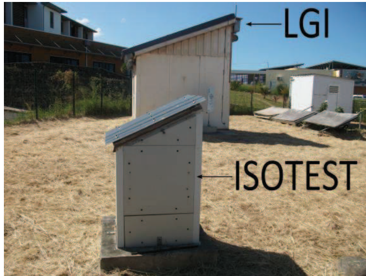
Figure 3: LGI and ISOTEST test cells
