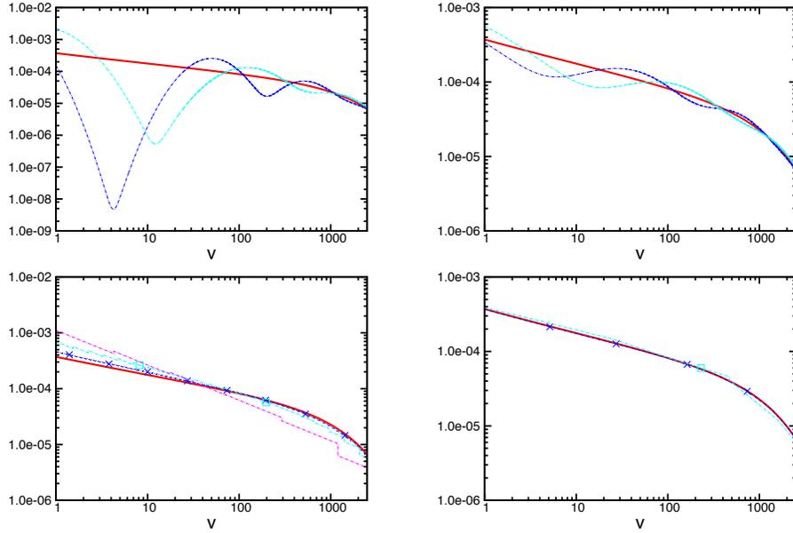
Figure 15: Reconstructed NDF at  $t = 6$ . Ln-EQMOM (left):  $N = 3$  (dashed cyan line) and  $N = 4$  (dashed blue line). Gamma-EQMOM (right):  $N = 3$  (dashed cyan line) and  $N = 4$  (dashed blue line). OSM (bottom left): 10 (dashed magenta line), 30 (dashed cyan line), 90 (dashed blue line) sections. TSM (bottom right): 5 (dashed cyan line), 15 (dashed magenta line), 45 (dashed blue line), 101 (red solid line).
