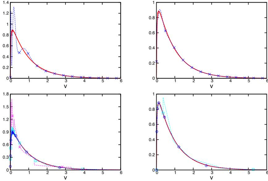
Figure 12: Brownian aggregation with self-similar NDF (red solid line). Ln-EQMOM (top left):  $N = 4$  (dashed blue line). Gamma-EQMOM (top right):  $N = 4$  (dashed blue line). OSM (bottom left) with 10 (dashed magenta line), 30 (dashed cyan line) and 90 (dashed blue line) sections. TSM (bottom right) with 5 (dashed cyan line), and 15 (dashed blue line) sections.
