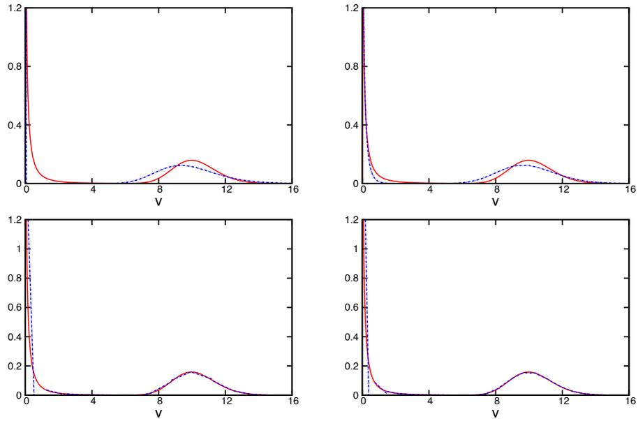
Figure 4: NDF at  $t = 0.033$  for size reduction using  $v$ -reconstruction: exact (solid red line) and numerical (dashed blue line) solutions. Ln-EQMOM  $N = 4$  (top left). Gamma-EQMOM  $N = 4$  (top right). TSM with 41 sections: CFL=0.9 (bottom left) and CFL=0.05 (bottom right).
