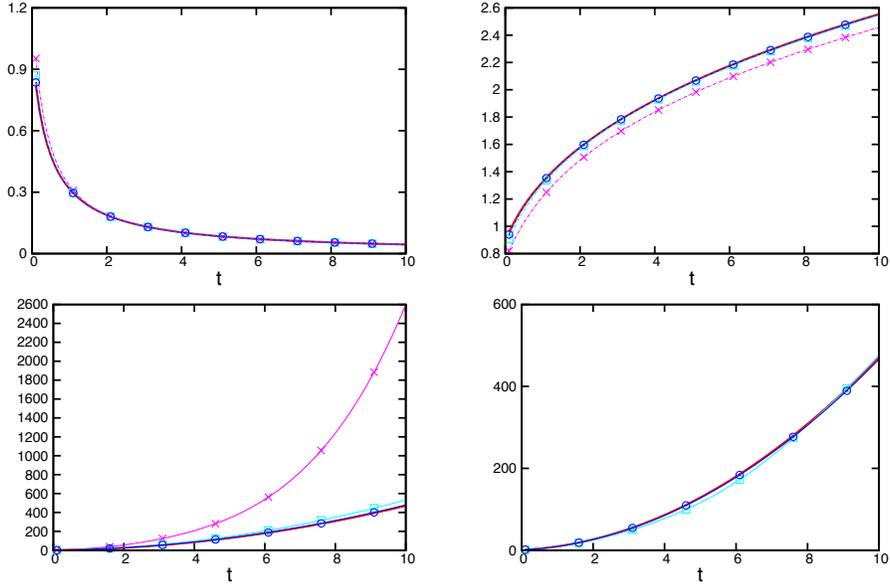
Figure 11: Brownian aggregation with self-similar NDF. Evolution of  $m_0$  (top left), mean particle diameter (top right) and variance (bottom) versus reference solution (red solid line). OSM (top, bottom left) with 10 (dashed magenta line), 30 (dashed cyan line) and 90 (dashed blue line) sections. TSM (bottom right) with 5 (dashed cyan line), and 15 (dashed blue line) sections.
