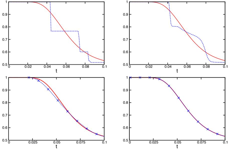
Figure 5: Evolution of  $m_0$  for size reduction using  $r$ -reconstruction: exact (solid red line) and numerical (dashed blue line) solutions. Ln-EQMOM  $N = 4$  (top left). Gamma-EQMOM  $N = 4$  (top right). TSM with 9 (bottom left) and 41 sections (bottom right).
