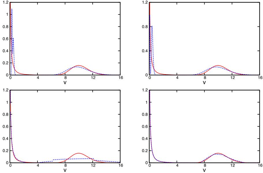
Figure 8: NDF at  $t = 0.033$  for size reduction using  $r$ -reconstruction: exact (solid red line) and numerical (dashed blue line) solution. Ln-EQMOM  $N = 4$  (top left). Gamma-EQMOM  $N = 4$  (top right). TSM with 9 (bottom left) or 41 (bottom right) sections.
