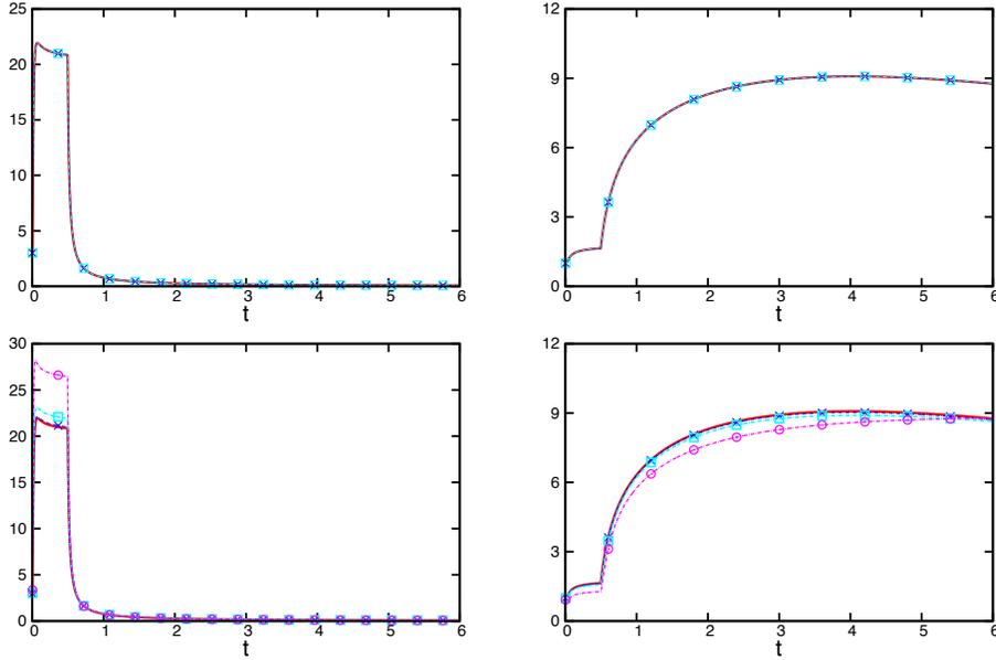
Figure 13: Time evolution of  $m_0$  (left) and mean particle diameter (right). Ln-EQMOM (top row):  $N = 3$  (dashed cyan line),  $N = 4$  (dashed blue line). OSM (bottom row): 10 (dashed magenta line), 30 (dashed cyan line), 90 (dashed blue line) sections. TSM, with 101 sections: (red solid line).
