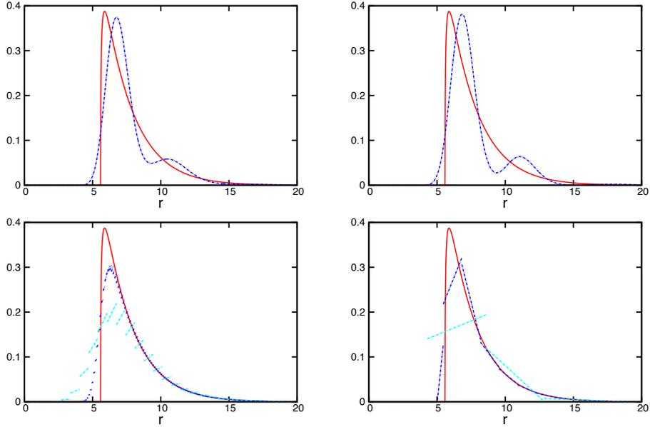
Figure 10: NDF for diffusion-controlled growth at  $t = 20$ : numerical (dashed blue line) vs. exact (solid red line). EQMOM reconstruction with  $r$ -moments,  $N = 4$ : Ln (top left), gamma (top right). OSM reconstruction (bottom left) with 90 (dashed cyan line) and 500 (dashed blue line) sections. TSM reconstruction (bottom right) with 15 (dashed cyan line) and 45 (dashed blue line) sections.
