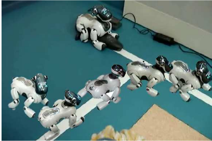
Fig. 4: The battery charging experiment.
