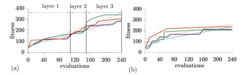
**Fig. 2.** Fitness values at each evaluation during USARSim training (solid lines: GA in blue, NM in green and PG in red) and linear interpolations (dashed lines): (a) incremental learning, (b) learning all parameters.
