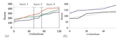
**Fig. 3.** Fitness values during AIBO training: (a) incremental learning (solid lines: GA in blue, NM in green, PG in red) with start point derived from USARSim, and linear interpolations (dashed lines), (b) comparing GA for  $L_1$ : with initial population derived from USARSim (solid blue line), and with random initial population (solid black line), and linear interpolations (dashed lines).
