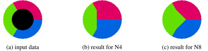
Figure 9: inpainting . Depicted above are solutions (b) and (c) of synthetic instances of the inpainting problem (a). It can be seen that discretization artifacts due to the 4-neighborhood (b) are smaller than discretization artifacts due to the 8-neighborhood (c).
