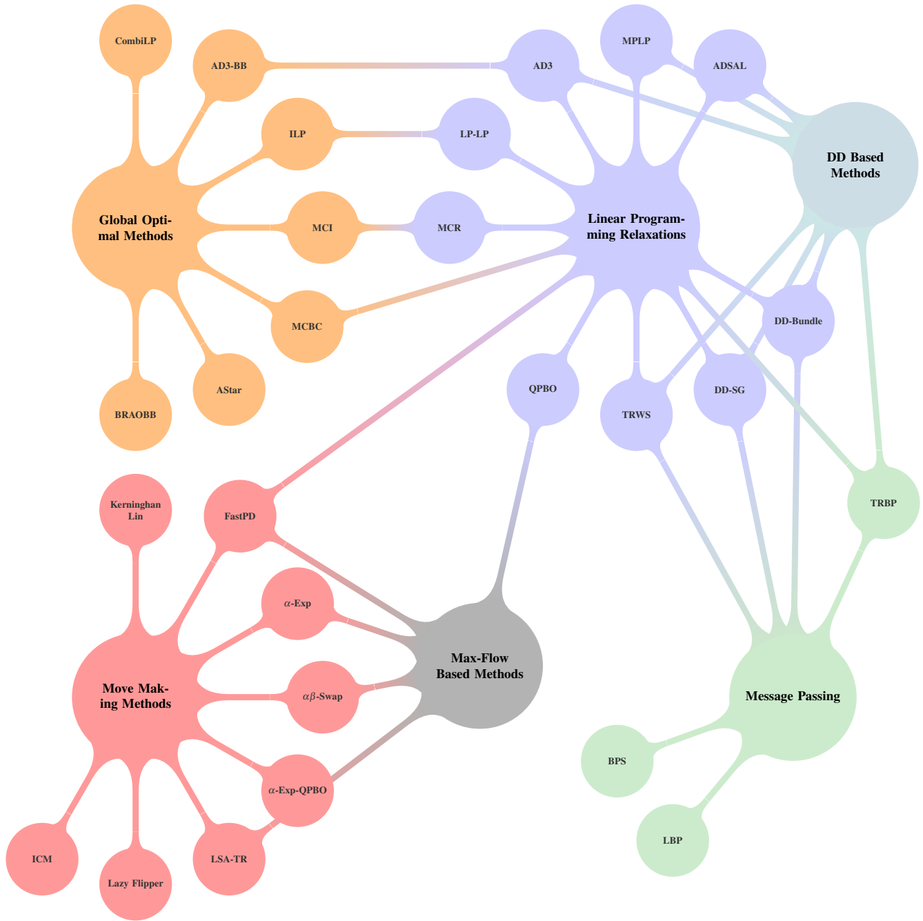
Figure 4: The inference methods used in this benchmark can be roughly grouped into four classes. These are (1) methods based on linear programming , (2) methods providing global optimal solutions, which are often strongly related to linear programming, (3) methods based on move-making procedures which iteratively improves the labeling, and (4) methods based on message passing – often motivated by linear programming and variational optimization. Some methods make use of max-flow methods for fast optimization of binary (sub-)problems or based on the dual decomposition framework, which is also sketched in the diagram. A fifth class of methods are methods based on sampling , which are not covered in this study since they are rarely used in computer vision. For hard models they might perform reasonable, with a certain amount of tuning of involved hyper-parameters and sampling procedures, as shown for the dtf-chinesechar model.
