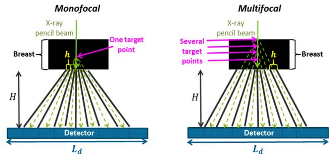
Fig. 2. Schematic representation of the two collimation systems.
