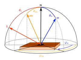
Figure 1: Geometry of reflection with our notation.
