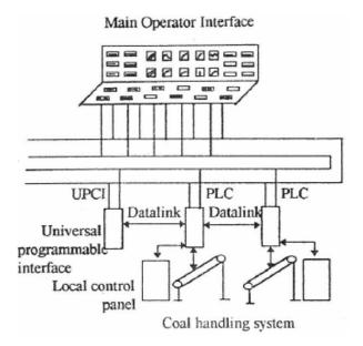
Fig. 3. PLC Control and DCS VDU/Local Control Panel Operator Interface
