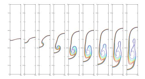
Figure 18: Rayleigh–Taylor instability. Simulation by the Hybrid FV-FE method, with the upwind scheme for the transport. Density contours  $2 \le \rho \le 4$  at times  $T=1,\,1.5,\,2,\,2.5,\,3,\,3.25,\,3.5,\,3.75$  and 4 (in Tryggvason's scale).
