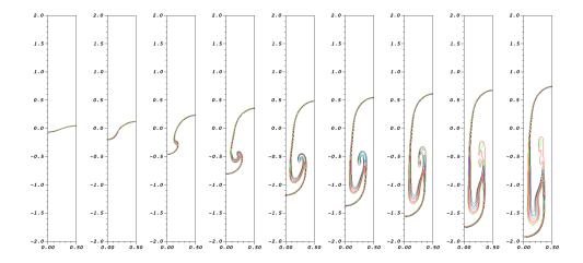
Figure 16: Rayleigh–Taylor instability. Simulation by the DDFV method. The dual mesh is constructed as in Figure 12. Density contours  $2 \le \rho \le 4$  at times  $T=1,\ 1.5,\ 2,\ 2.5,\ 3,\ 3.25,\ 3.5,\ 3.75$  and 4 (in Tryggvason's scale).
