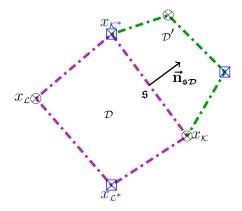
Figure 8: The definition of the gradient on the diamond mesh uses the unknowns stored at the nodes  $x_{\kappa}, x_{\varepsilon}, x_{\kappa^*}, x_{\varepsilon^*}$ .
