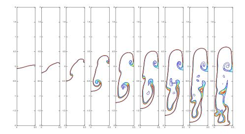
Figure 13: Rayleigh–Taylor instability. Simulation by the Hybrid FV-FE method, MUSCL scheme that degenerates at the boundary. Density contours  $2 \le \rho \le 4$  at times T = 1, 1.5, 2, 2.5, 3, 3.25, 3.5, 3.75 and 4 (in Tryggvason's scale).
