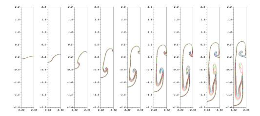
Figure 17: Rayleigh–Taylor instability. Simulation by the DDFV method. The dual mesh is constructed as in Figure 15. Density contours  $2 \le \rho \le 4$  at times T = 1, 1.5, 2, 2.5, 3, 3.25, 3.5, 3.75 and 4 (in Tryggvason's scale).
