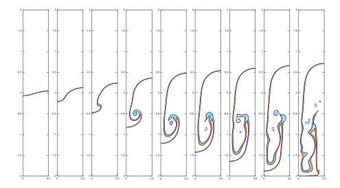
Figure 14: Rayleigh–Taylor instability. Simulation by the Hybrid FV-FE method, MUSCL scheme with "ghost cells" for the boundary. Density contours  $2 \le \rho \le 4$  at times T=1, 1.5, 2, 2.5, 3, 3.25, 3.5, 3.75 and 4 (in Tryggvason's scale).
