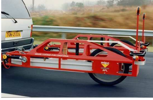
Fig. 6. LCPC laboratory vehicle towing LPA (Imine et al. (2006)).
