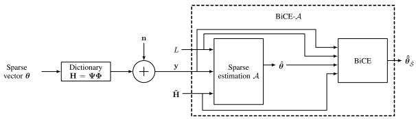
Fig. 1. Description of the BiCE-A. Note that algorithm  $A(\cdot)$  stands for any sparse-based estimators.
