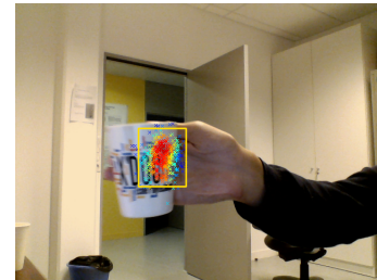
Fig. 2. Particle Filter used alone. Each coloured pixel corresponds to the projection of the particle in the spatial space. Its colour represents its weight (Equation 2): red corresponding to high weight, blue to low weight. The rectangle is the state estimated with the Particle Filter, processed alone, using the equation 3. Its colour corresponds to the weight of the observation, for its state.
