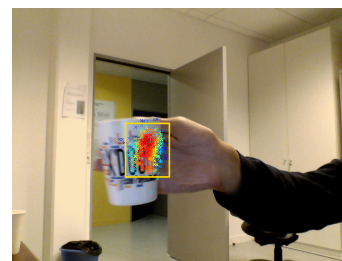
Fig. 2. Particle Filter used alone. Each coloured pixel corresponds to the projection of the particle in the spatial space. Its colour represents its weight (Equation 2): red corresponding to high weight, blue to low weight. The rectangle is the state estimated with the Particle Filter, processed alone, using the equation 3. Its colour corresponds to the weight of the observation, for its state.
