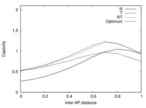
Fig. 8. Capacity with respect to inter-AP distance for two frequency channels.
