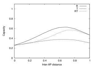
Fig. 7. Capacity with respect to inter-AP distance for a single frequency channel.
