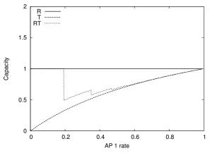
Fig. 2. Capacity with respect to AP-1 rate  $R_1$  for a single frequency channel when  $R_2 = 1$ .
