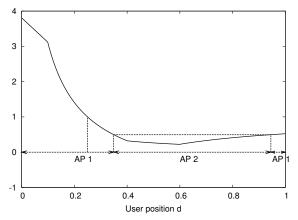
Fig. 9. Ratio of physical rates  $R_1(d)/R_2(|d-D|)$  for D = 0.5.
