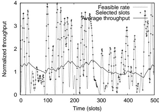
Figure 5: The SB scheduler with rate constraints.
