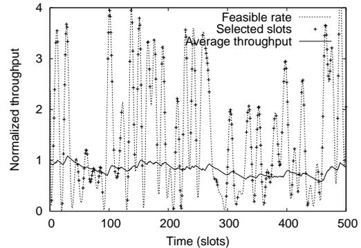
Figure 2: The PF scheduler with rate constraints.
