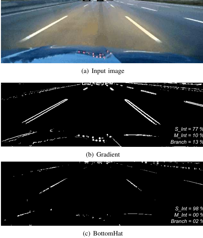
Figure 5. Successive steps of the lane detection application, and their computing profile.
