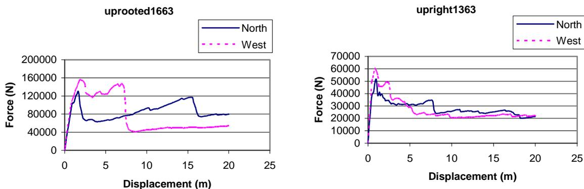
Fig. 6: two examples of force vs. displacement curves showing anisotropic responses and hardening.
