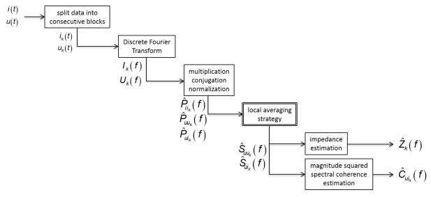
Figure 3: Frequency evolutionary impedance estimation method.
