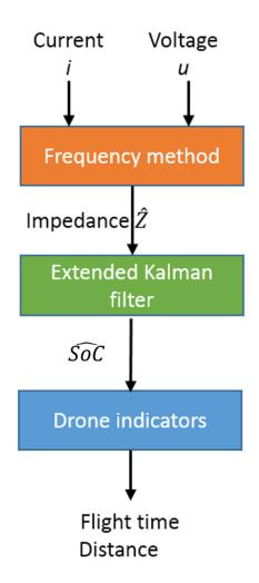
Figure 12: Algorithm to estimate the SoC and the remaining flight time and distance.
