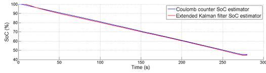
Figure 13: SoC estimation by Coulomb counter and EKF.
