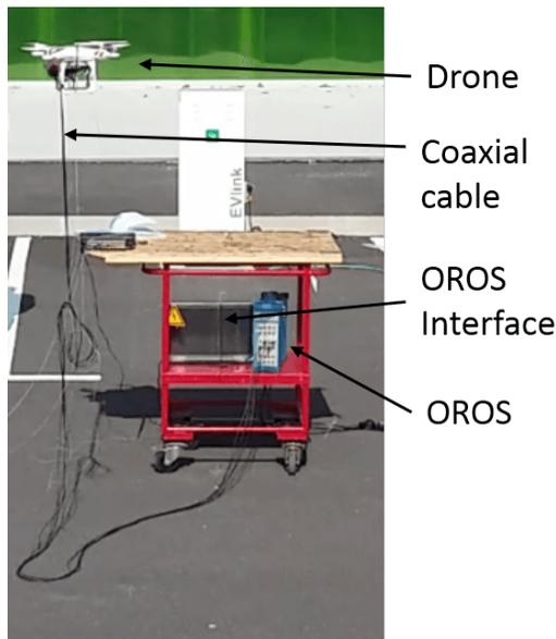
Figure 5: Drone experimentation device.
