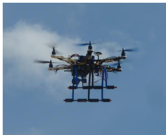
Figure 2: The UAV used during the flights, based on a modify F550 DJI frame.
