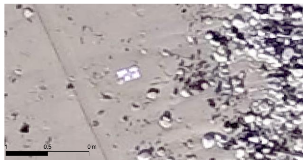
Figure 3: Ortho Image (3 cm pixel size) of a GCP and its target paper.
