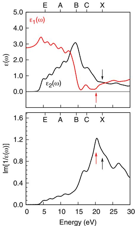
FIG. 10. (Color online) Cubane optical properties: Top panel: Real (red) and imaginary (black) parts of the dielectric tensor in RPA +  $G_0W_0$ . Bottom panel: Electron energy-loss spectrum at vanishing momentum. Red and black arrows mark the positions of the first minimum of  $\epsilon_1(\omega)$  and of the X transition, respectively.
