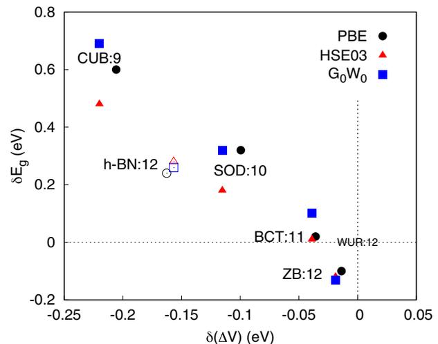
FIG. 5. (Color online) Variations of the gap widths  $\delta E_g$  versus the variation of electrostatic potential difference  $\delta(\Delta V)$ , with respect to the gap and potentials in the wurtzite structure. Results obtained within the PBE, HSE03, and  $G_0W_0$  approximations are represented with black dots, red triangles, and blue squares, respectively.  $N_2$  values are also reported for each structure.
