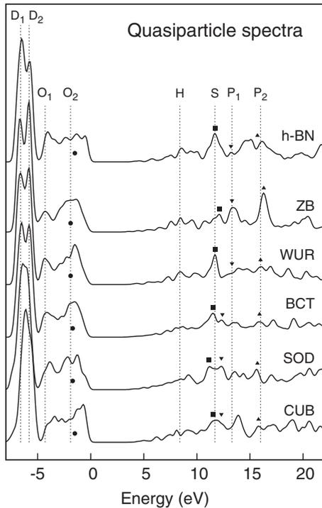
FIG. 6.  $G_0W_0$  total density of states (arbitrary units) of the six ZnO polymorphs aligned at the top of the VB. Black round dots mark the center of gravity of the  $O_2$  region, squares mark the position of the highest peak of Zn  $4s$  character, and down-pointing and up-pointing triangles mark the position of the  $P_1$  and  $P_2$  regions respectively. Vertical lines indicate the positions of the main wurtzite structures as a guide for the eyes.
