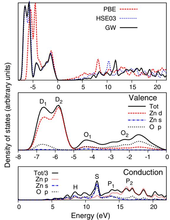
FIG. 4. (Color online) Top panel: ZnO wurtzite total DOS, calculated within PBE (red dashed), HSE03 (blue dotted), and  $G_0W_0$  (black solid) approaches. Central panel: Atom- and orbital-projected  $G_0W_0$  DOSs in the VB. Bottom panel: Atom- and orbital-projected  $G_0W_0$  DOSs in the CB. All curves are aligned at the valence band maximum.
