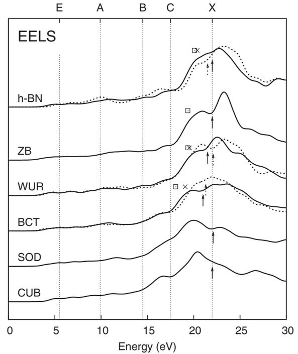
FIG. 9. EELS spectra of the six ZnO polymorphs. OCs (parallel) and ECs (perpendicular) spectra are reported with solid and dashed lines, respectively. Squares and  $\times$  signs mark the energies where  $\epsilon_1(\omega) = 0$  for OCs and ECs. An arrow indicates the position of the X structure. The positions of wurtzite peaks E, A, B, C, and X are indicated by vertical lines to guide the eye.
