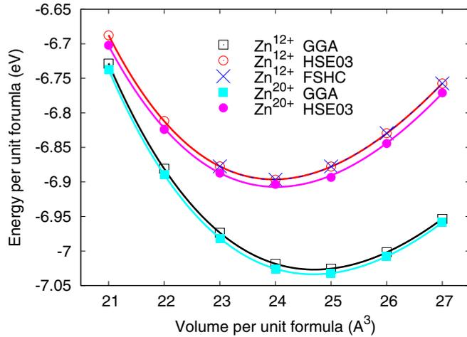
FIG. 1. (Color online) Wurtzite energy versus volume  $E(V)$  curves, computed with PBE (generalised gradient approximation GGA) and HSE03 XC functionals and the FSHC scheme (see text), in which the core electrons are represented by the  $\text{Zn}^{12+}$  or  $\text{Zn}^{20+}$  pseudopotential.
