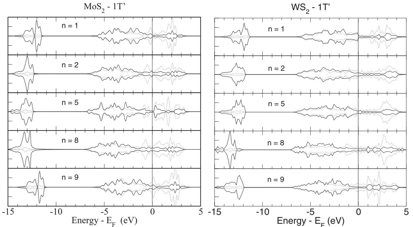
FIG. 6. Row-projected densities of states across  $1T'$   $N = 9$  nanoribbons. Left:  $MoS_2$ , right:  $WS_2$ . Rows 3 and 4 and 6 and 7 are skipped for simplicity. The Fermi level is at zero energy. Solid (dotted) lines correspond to S (Mo/W) projections.
