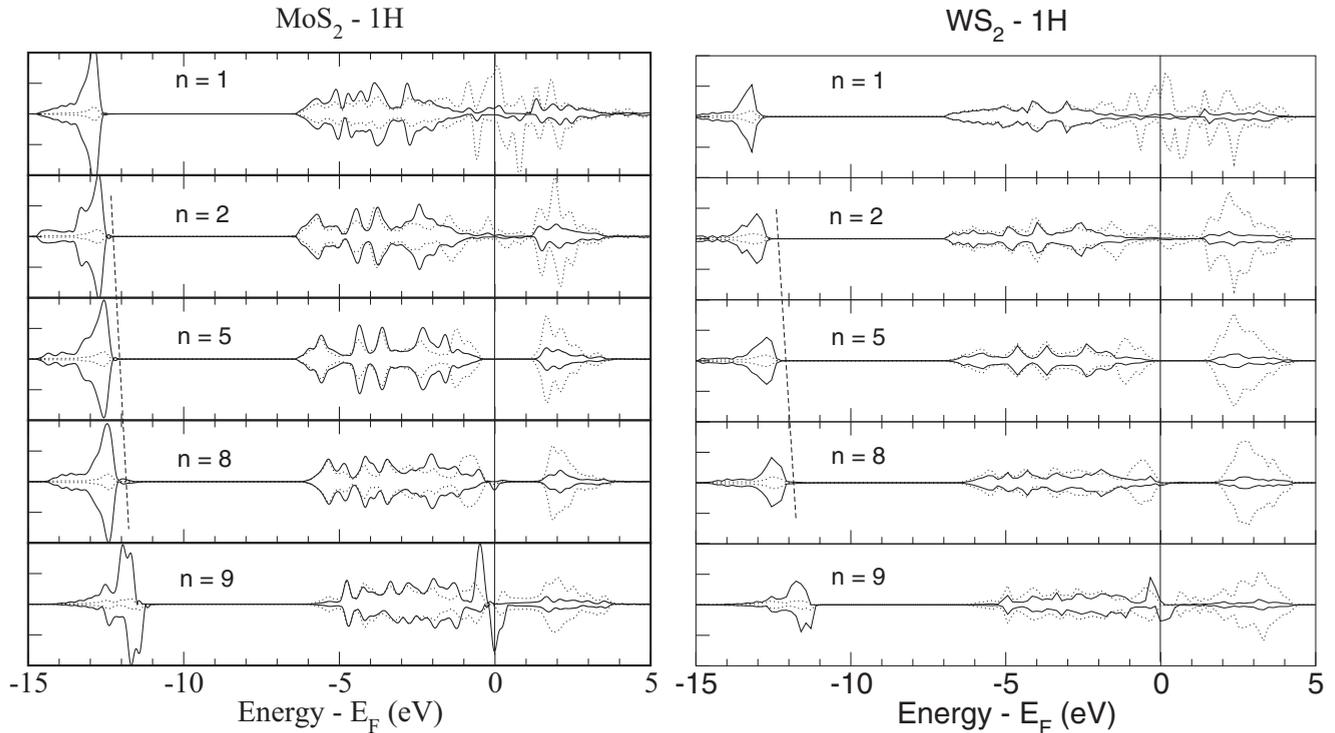
FIG. 4. Row-projected densities of states across 1H  $N = 9$  nanoribbons. Left: MoS<sub>2</sub>, right: WS<sub>2</sub>. Rows 3 and 4 and 6 and 7 are skipped for simplicity. The Fermi level is at zero energy. Solid (dotted) lines correspond to S (Mo/W) projections. The dashed line is a guide for the eyes and shows the shift of the semicore S states across the ribbon.
