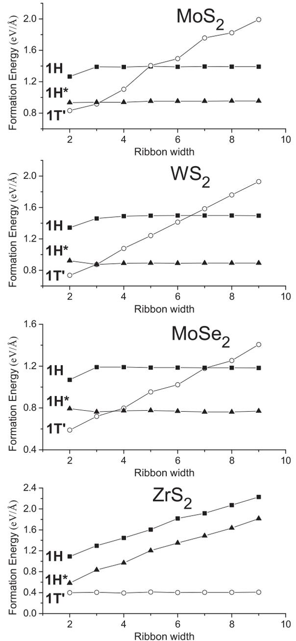
FIG. 3. From top to bottom, formation energies per unit length of  $\text{MoS}_2$ ,  $\text{WS}_2$ ,  $\text{MoSe}_2$ , and  $\text{ZrS}_2$  1H (filled squares), 1H\* (filled triangles) and 1T' (open circles) ribbons, as a function of ribbon width.
