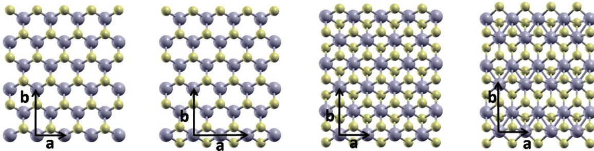
FIG. 1. (Color online) From left to right, top view of 1H, 1H\*, 1T, and 1T' MoS<sub>2</sub> monolayers/ribbons: Mo (gray) and S (yellow). Rectangular unit cell vectors are explicitly plotted. If the structures shown are considered periodic only in the  $a$  direction, they correspond to the  $N = 6$  zigzag nanoribbons. In the 1H\* ribbons, the unit cell vector  $a$  is doubled due to a different relaxation of neighboring edge atoms.
