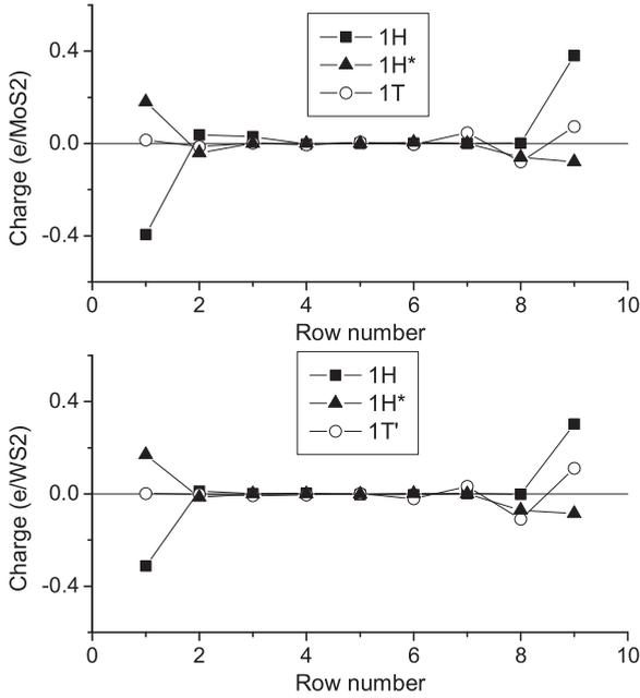
FIG. 7. Values of row projected Bader charge modifications with respect to central row of the  $N = 9$  nanoribbons. Top: MoS<sub>2</sub>; bottom: WS<sub>2</sub>.
