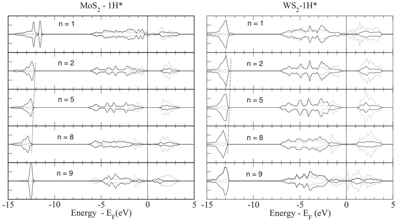
FIG. 5. Row-projected densities of states across  $1H^*$   $N = 9$  nanoribbons. Left:  $MoS_2$ , right:  $WS_2$ . Rows 3 and 4 and 6 and 7 are skipped for simplicity. The Fermi level is at zero energy. Solid (dotted) lines correspond to S (Mo/W) projections. The dashed line is a guide for the eyes and shows the shift of the semicore S states across the ribbon.
