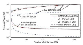
Fig. 8. Total PA power at the EE-maximizing solution for different number of BS antennas in the single-cell scenario. The radiated power per BS antenna is also shown.
