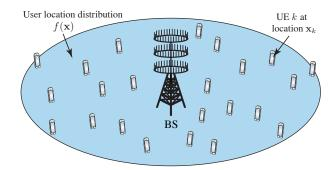
Fig. 2. Illustration of a generic multi-user MIMO scenario: A BS with M omnidirectional antennas communicates with K single-antenna UEs in the uplink and downlink. The user locations are selected from an arbitrary random user distribution  $f(\mathbf{x})$ .
