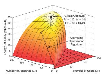
Fig. 3. Energy efficiency (in Mbit/Joule) with ZF processing in the singlecell scenario. The global optimum is star-marked and the surroundings are white. The convergence of the proposed alternating optimization algorithm is indicated with circles.
