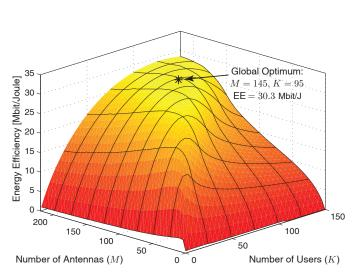
Fig. 4. Energy efficiency (in Mbit/Joule) with MMSE processing in the singlecell scenario.
