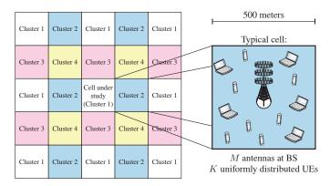
Fig. 10. The multi-cell simulation scenario where the cell under study is surrounded by 24 identical cells. The cells are clustered to enable different pilot reuse factors.
