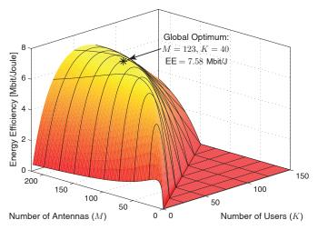
Fig. 14. Energy efficiency (in Mbit/Joule) with ZF processing in the multi-cell scenario with pilot reuse 4.
