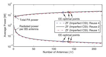
Fig. 12. Total PA power at the EE-maximizing solution in the multi-cell scenario, for different number of BS antennas. The radiated power per BS antenna is also shown.
