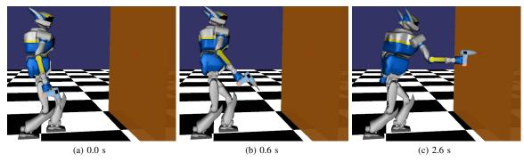
Fig. 11. Test 5. Snapshots of the drilling task. The red dot on the wall represents the desired hole position.
