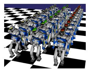
Fig. 1. Simulation of 30 HRP-2 robots walking in the presence of uncertainties, the goal being to compare the classic TSID controller (left line, gray heads) to the proposed robust TSID controllers: stochastic (central line, green heads) and worst-case (right line, red heads). Some of the simulation results can be seen in the accompanying video.
