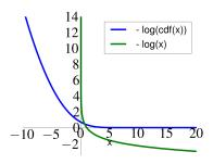
Fig. 5. Comparison of the logarithmic barrier used in (15) with the barrier used in (14). For the plot we considered a standard deviation of 2.0 for the CDE
