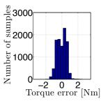
(a) Hip pitch joint, left front leg, mean 0.15 Nm, standard deviation 0.8 Nm.
