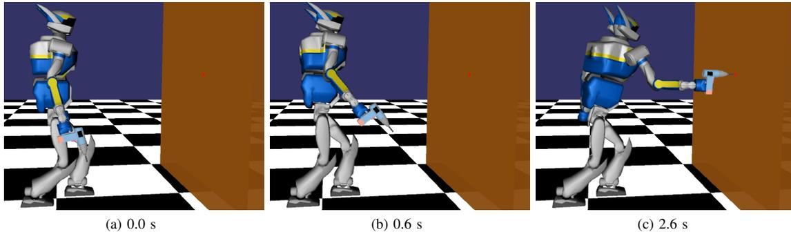
Fig. 11. Test 5. Snapshots of the drilling task. The red dot on the wall represents the desired hole position.
