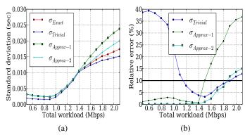
Figure 2: (a) Exact vs Approximate solutions for the standard deviation of the end-to-end delay. (b) Relative error committed by the approximate solutions.
