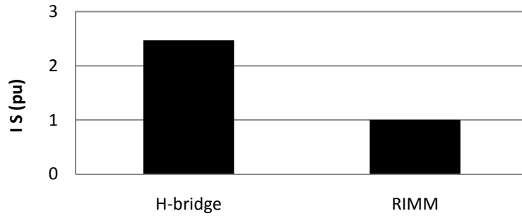
Fig. 11: Inverter sizing of both topologies
