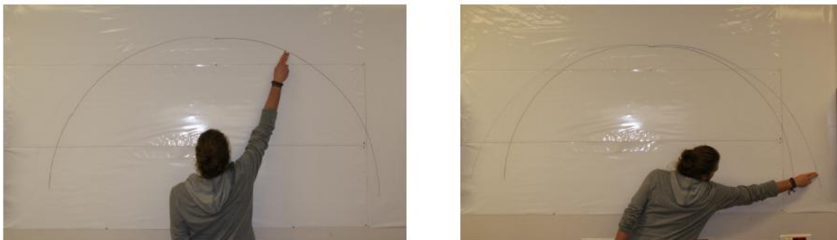
Figure 5. Continuous experimental test B1 (left) with the feet and the body fixed, and test B2 (right) with the feet fixed and the upper body in movement.
