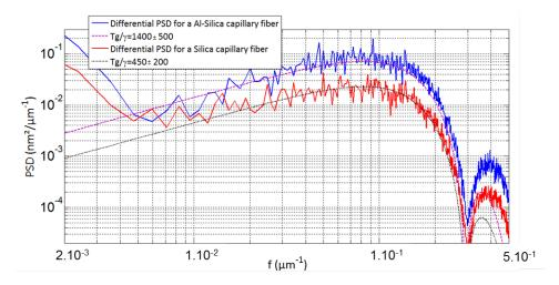
Fig. 6. Differential profilometry measurements on inner surfaces of two hollow glass fibres (silica and alumina doped silica). The power spectral densities of the differential height signal are represented as continuous lines. The dashed lines are fits obtained with the analytical expression (16). The linear trend observed at low frequency is consistent with a scenario of frozen capillary waves at the glass surface.
