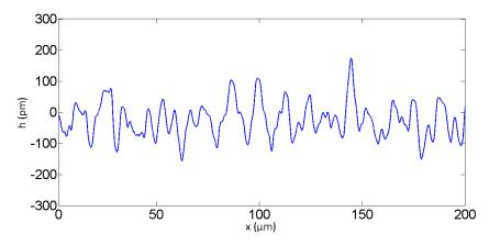
Fig. 5. Differential profile obtained on the inner surface of a silica capillary tube over a length of 200  $\mu$ m. Height fluctuations are extremely low, in the range of a few hundreds of picometers.
