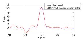
Fig. 4. Tests on silica steps obtained in air by RIE etching (exposure time 15s). Left: AFM image (estimated step height 11.7nm) Right: Differential profilomety measurement obtained at the glass/air interface on the same step (estimated step height 11.1nm after fitting with analytical expression (5), using  $d = 6.5 \mu m$  and  $w = 2.0 \mu m$ ). The displacement step size used for the measurement was  $0.18 \mu m$ .
