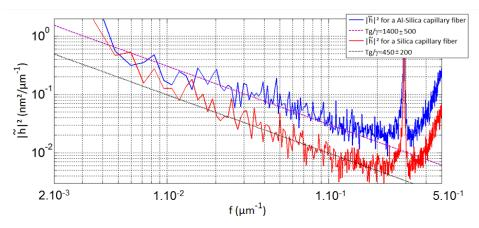
Fig. 7. Roughness measurements on inner surfaces of two hollow glass fibres (silica and alumina doped silica). The power spectral densities of the height signal are obtained after division by the response function. The dashed and dotted lines are fits obtained with the analytical expression (15). The clear 1/f trend observed at low frequency is consistent with a scenario of frozen capillary waves at the glass surface.
