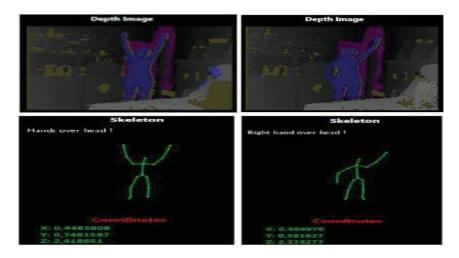
Fig. 13.Gesture recognition using Kinect
