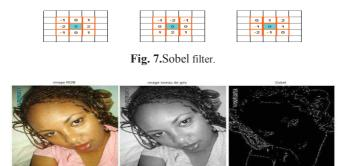
Fig. 8. Example of edge detection using the Sobel filter
