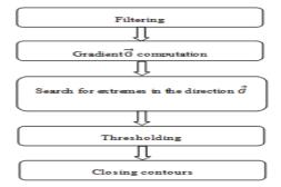
Fig. 5.Flow chart of the Gradient Approach
